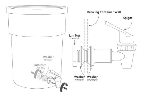
Screw the spigot, the inside & outside washers, and the jam nut together through the hole in the brewing container wall.
