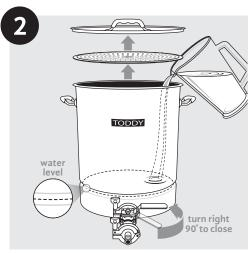
**Step 2** Close the valve completely. Remove filter platform and add a portion of the filtered water to fill the brewer to the middle of the support ring.
