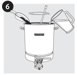
Step 6 Carefully stir with a mixing paddle, avoiding contact with the filter. Repeat step 5 to add the remaining coffee and filtered water. Tip: For best results, mix coffee grounds by pulling and plunging them from the edge of the brewer toward the center.
