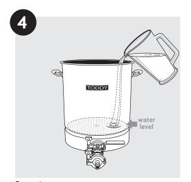
Step 4 Slowly add just enough water to wet the filter and fully submerge.
