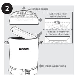
Step 2 Slide the platform into a new filter, and fold as indicated above. Holding the bridge handle insert the platform and filter, guiding the platform into place until it rests on the support ring.
