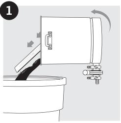
**Step 1** Using a *team lift*, invert the brewer over a waste or compost bin to remove all coffee grounds and filter platform.
