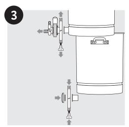
**Step 3** Remove the valve and attach cleaning blank to the flange using a clean gasket and a tri-clamp.
