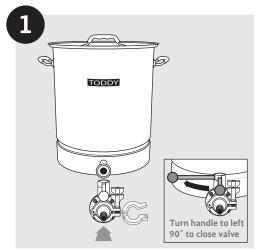
**Step 1** Install valve assembly so the handle points away from the system when the valve is open. Tip: To turn the valve handle, pull out on the handle. Close the valve completely. Set aside the cleaning blank.
